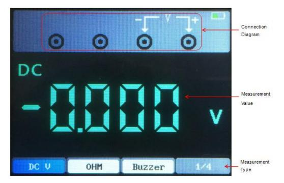
The measuring types include DC voltage (V, mV), AC voltage, DC current (A, mA), AC current (A, mA), resistance, capacitance, diode, and on-off test.
